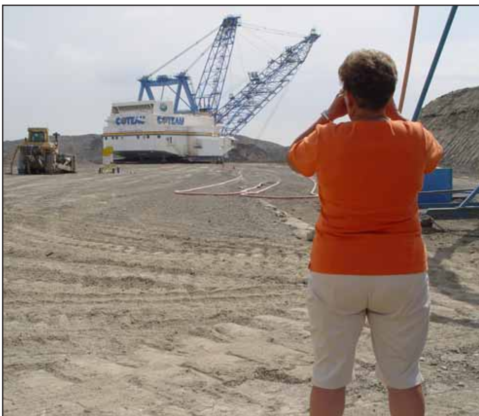
An electric cooperative member snaps a photo of the huge dragline which uncovers lignite coal near Antelope Valley Station in North Dakota, one of several coal-fired generating stations providing power to NIPCO-area cooperative members.
